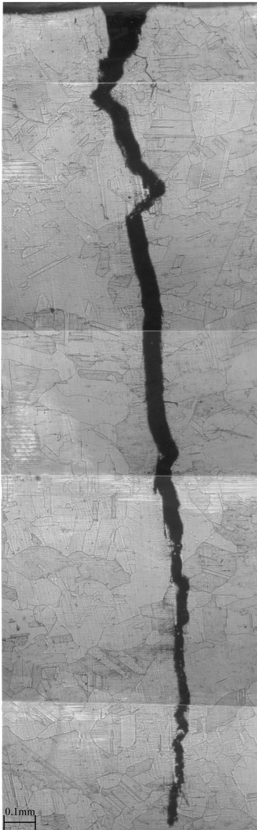
Fig. 3—Optical micrograph of the cross section of the mold crack.
